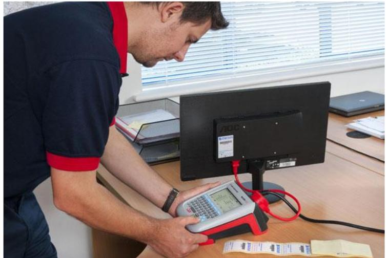
An important factor in the company's choice of the new tester is the inclusion of an integrated digital camera for the visual inspection of appliances and an expanded internal memory that means all test results can be recorded automatically for downloading to results databases.
