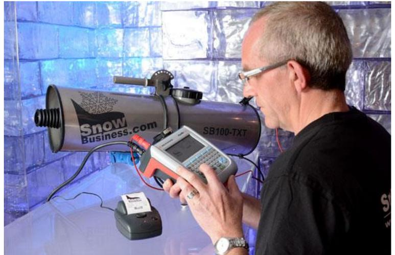
Among the wide range of equipment tested are special falling snow machines, snow 'blower' generators and agitators, high pressure pumps and associated extension cables, RCDs and electrical accessories.
