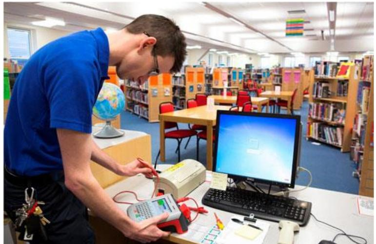
The focal point of the school's portable appliance testing policy is a Seaward Apollo 600 tester. This multi-purpose PAT tester combines electrical testing with sophisticated safety data collection features, including an onboard digital camera, to help those involved in maintaining safety in the workplace to demonstrate compliance with all the latest guidance on inspection and testing programmes.
