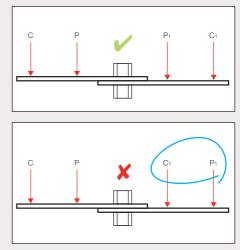
Measurement of joint resistance of 2 busbars
