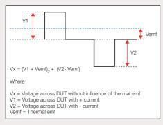
The second method sometimes employed is to connect the current terminals of the ohmmeter together, and with the potential leads connected to the DUT, measure any thermal emf that may be present. This measured value is then stored and deducted from the next measurement with current and potential leads connected to the DUT in the normal way. This is all done automatically when using Cropico Ohmmeters in the auto zero mode.
