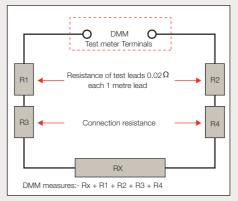
When measuring larger resistance values this additional lead resistance error can be ignored, but as you can see from the chart below, the error becomes significantly higher as the measured value decreases, and totally inappropriate below  $10\Omega$ .
