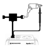
The External Leakage Adaptor test function, on the Apollo+ Series, is intended to be used only in conjunction with the one of Seaward's External Leakage Adaptors.
