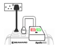
The Apollo+ Series should be connected to a mains supply. The RCD should be plugged into the EUT test socket (on the Apollo+ Series) and a connection should be made from the RCD mains output to the IEC test socket.
