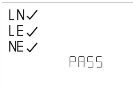
If the Live and Neutral in the socket wiring are reversed or there is a fault with the protective earth connection this is indicated by the display below.
